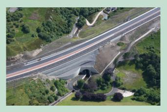
Macrete manufactured and supplied over 17,000m<sup>2</sup> of precast reinforced earth facing panels to the long-term construction of the A465 in North Wales.
